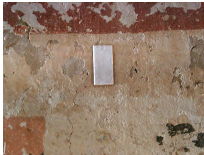
FIGURE 3 Prewetted paper strip applied to a wall painting in cave 85.
