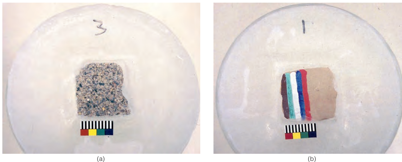
FIGURE 6 Sodium chloride migration experiments. (a) Conglomerate; (b) conglomerate with a layer of clay plaster, half of upper surface painted with pigments found at Mogao.
