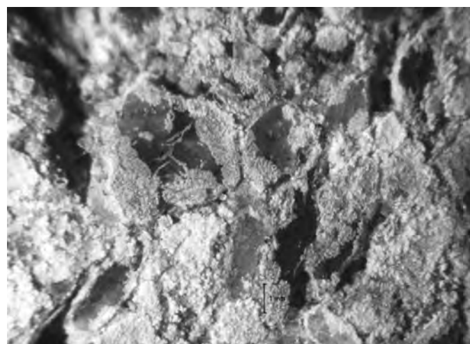
FIGURE 7 Sodium chloride crystallization on upper surface of conglomerate. Note salt creep around edges of larger grains.
