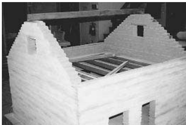
Figure 5.2 Model 8 before roof framing was added, with ridge beam in place.
