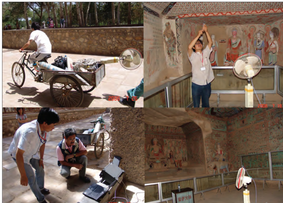
Fig. 6. Natural ventilation is measured by mixing a tracer gas ( \text{SF}_6 ) with cave air and measuring its dilution over time. The rate depends on a number of factors (open or closed doors; outside temperature and wind, cave size and configuration).
